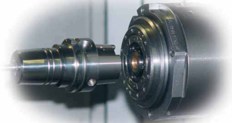
Fig. 1: HSK-A 63 interface, automatic tool change
