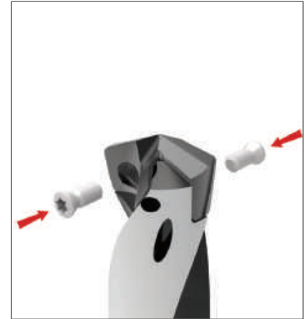
Step 3: Apply a generous amount of E-Z Break® (provided in the packaging) onto the supplied TORX® Plus screws.
