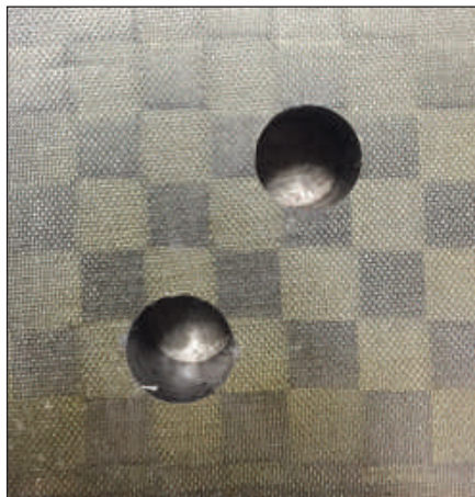
Holes drilled with PCD tooling
